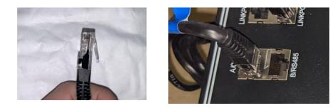
3. Install and fit the Can Com Cables by pressing and holding the plastic tab of the Can Com Cable in its respective ports. ACAN port for the battery and CAN Port for Inverter. (Please take note of the labels of the Cables in which port it will go to).
