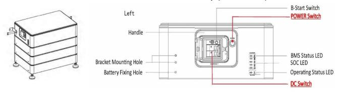
2) Turn off the battery <u>DC switch</u> also located on the control unit to the side of the master battery. (shown above)
